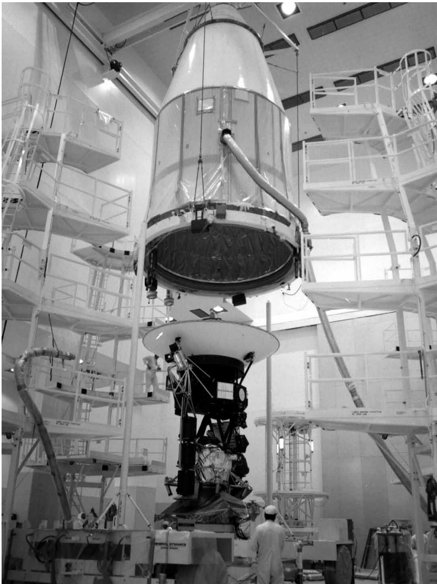
The Voyager 2 spacecraft, which was the first of the two Voyagers to launch, is seen at the Spacecraft Assembly and Encapsulation Facility 1 at NASA's Kennedy Space Center in Cape Canaveral, Florida. This archival photo is from August 1977. The spacecraft was put into this shroud on August 2, 1977, to protect it during flight through the atmosphere. Photo NASA/JPL-Caltech, NASA/JPL-Caltech Photojournal
